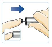
**STEP 4** Insert cartridge, threaded end first
